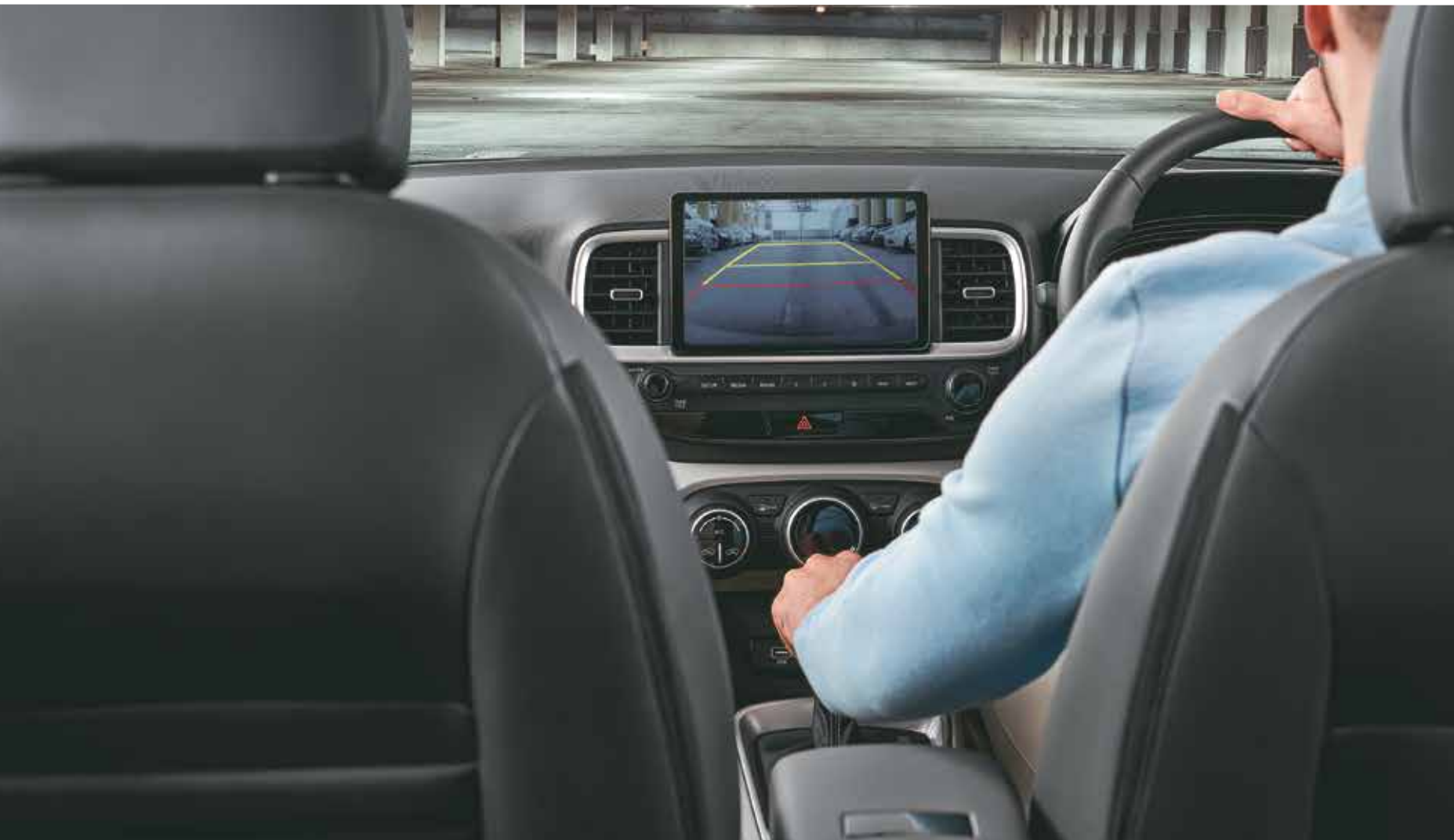
Rear parking assist camera with dynamic guidelines
